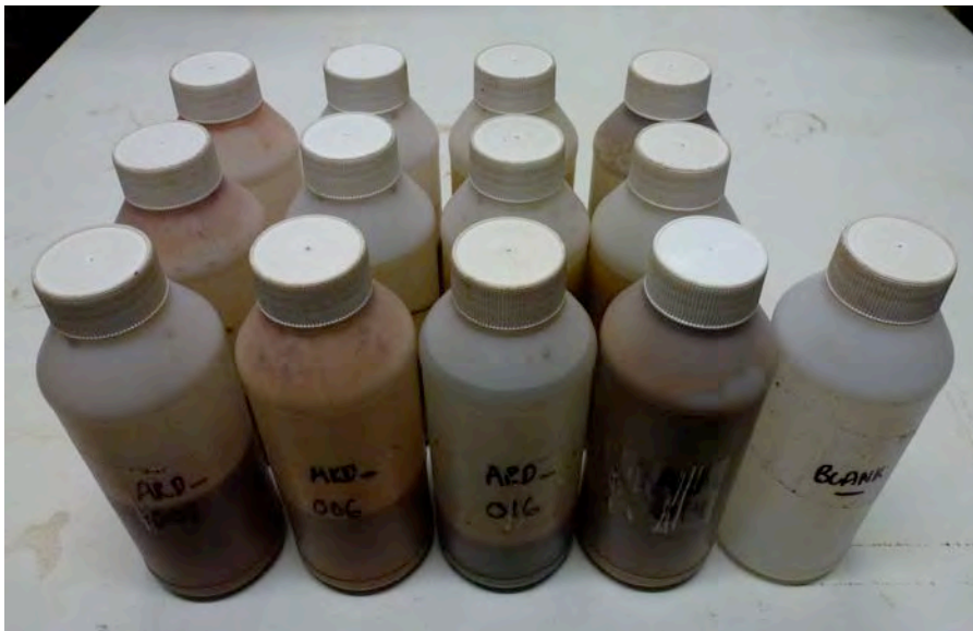
PLATE 6: Water-Extraction Testwork using 'coarse-crushings' (-5 mm nominal), and a solid:deionised-water ratio of 1:2 (w/w). Test-slurries agitated continuously via bottle-rolling, and then left to 'still-stand' for 1-2 days to allow 'fine-particulates' to settle, prior to decanting via siphoning. The decanted supernatants were then vacuum-filtered (0.45 \mu m-membrane), and resulting filtrates preserved, as appropriate, for specific analytes. Centrifugation at ca. 3,000 G for 30 mins was required for some samples to facilitate vacuum-filtration (see PLATE 7).
