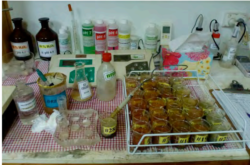
PLATE 2: Determination of pH-(1:2) and EC-(1:2) values (EC = Electrical-Conductivity) using crushings (-5 mm nominal). Test-slurries aged in contact with air at room-temperature (20-22 °C) for ca. 2-3 days prior to measuring pH and EC. The test-slurries were stirred using a spatula a number of times during this ageing period. Supernatant-water initially decanted for EC determination, and following return to beaker, slurry-pH measured. For a number of samples, the 'turbid/muddy' supernatants needed to be centrifuged at 3,000 G for 30 minutes in order to obtain clear supernatants suitable for EC measurement (see further below).
