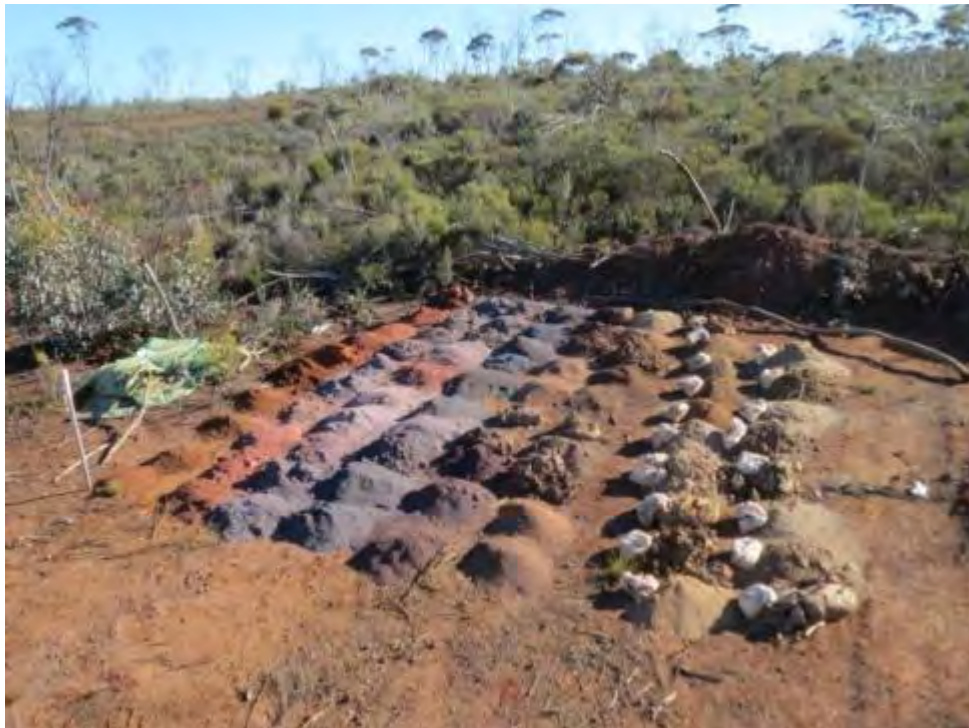
Figure 15. RC drillhole MRC008, Weathering and water table
