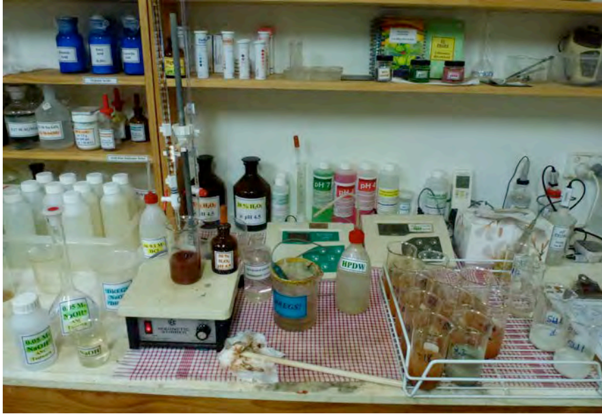
PLATE 5: Acid-Neutralisation-Capacity (ANC) testing using 'fine-crushings' (-2 mm, dry-sieved).
